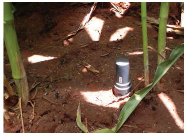
Above: DACOM soil moisture probe in maize field (© WRP (Pty) Ltd)
