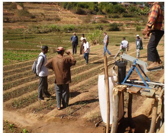
Above: Example of an MIS system: treadle pump, 100 litre bag and micro irrigation tubes (© AVSF)
