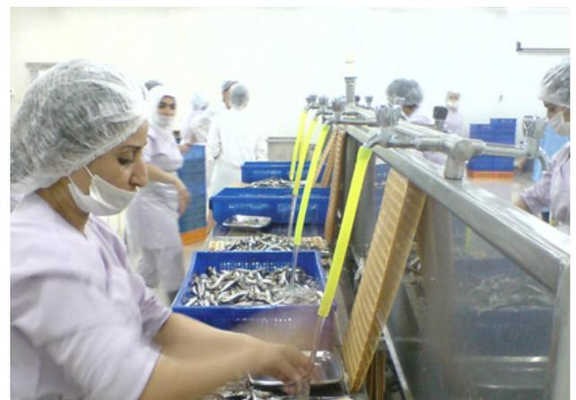
Above: New thawing system and anchovy gutting/filleting line
